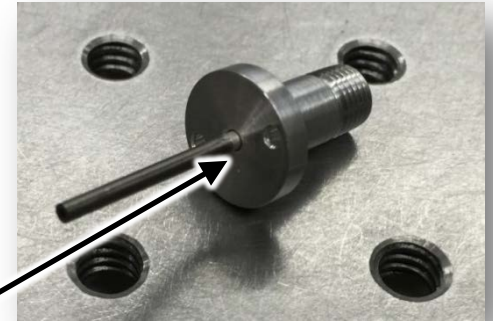
UV injector (Ti ferrule + UV fiber + SMA connector)
